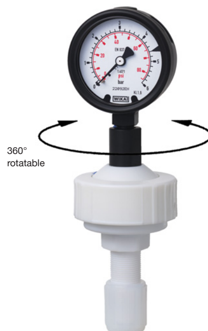
HYDRA-line Model HG, 63 mm gauge stainless steel series with black Teflon® coating and dead-end 1/2" flare process connection
